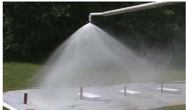
Outdoor test of wind drift effect on fire protection nozzles' spray coverage.
