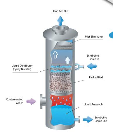
Drop size and atomisation is not top priority with a packed bed scrubber. Ensuring the fluid reaches over the top of the bed is the main objective as this will lead to good interaction as it evenly trickles down throughout the entire bed.
