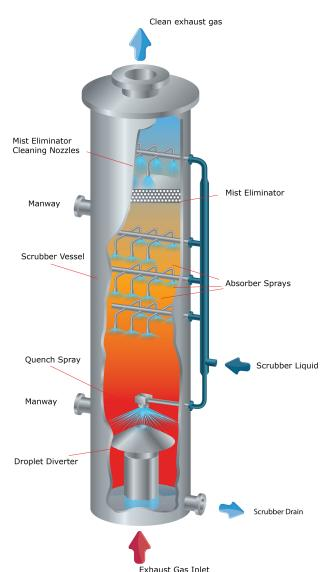
The basic operating principle of a wet scrubber is to pass a gas flow through an atomised spray which then interacts with the gas flow and knocks out contaminants.
