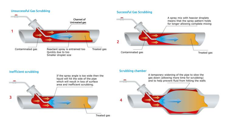
However, there is a lot more to consider than this; finely atomised sprays do produce much greater surface areas, but the light drops also get rapidly entrained in gas flows. Therefore, they are not able to reach the outer parts of a fast moving gas flow and parts of the gas will not come into contact with any of the reagents at all. Parts of the gas are going to be missed.
