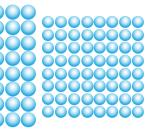
As a volume of water is broken into smaller and smaller droplets, the surface area increases. Drop size is what dictates the overall surface area of the spray.
