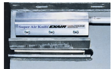
With a 40:1 air amplification ratio, a high volume of airflow is the result from minimal air input to keep linear induction motors from overheating.
