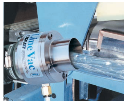
A Model 6084 2" (51mm) Line Vac transports scrap cellophane trim to a waste barrel.
