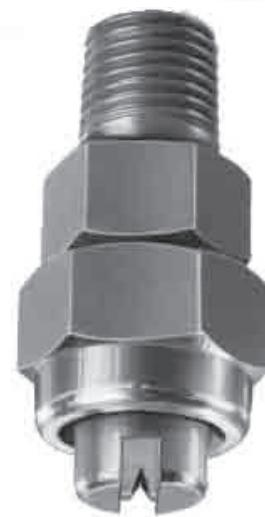
The BJ spray nozzle range is a low flow rate flat fan nozzle. It consists of three parts with a base, a spray tip and a cap nut (with an optional strainer). The base units and caps are universal meaning that spray tips can be swapped between base units.
