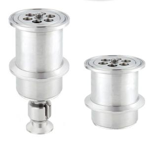
The EK is used in conjunction with a primary tank cleaner which will sit at the top of the tank above the product line. The EK will be positioned below the product line. The nozzle has two rotating fan jets giving 270° coverage side to side, making it ideal for spot cleaning difficult to reach areas.
