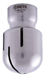
The HWS2 tank cleaning head delivers a robust cleaning action to the entire vessel. It is fluid powered, with the rotary action driven by liquid pressure.
