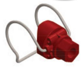
The MK2 nozzle holder is a handy way to attach spray nozzles to pipe work. The holder clamps around the pipe and a spigot with an o-ring inserts into a pre-drilled hole in the pipe. This attaches the clamp holder and forms a seal suitable for liquid pressures up to 4 bar (6 bar for the double clamp). The holder has a female thread to take any threaded nozzle. This product eliminates the need for threads to be tapped into pipe work, saving time and money.
