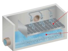
Jet cleaners activate, rotating on two axes. Powerful jets are brought to bear on each part of the screen
